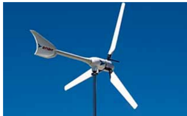
3,5 kW wind turbine in Castalla (Alicante)
